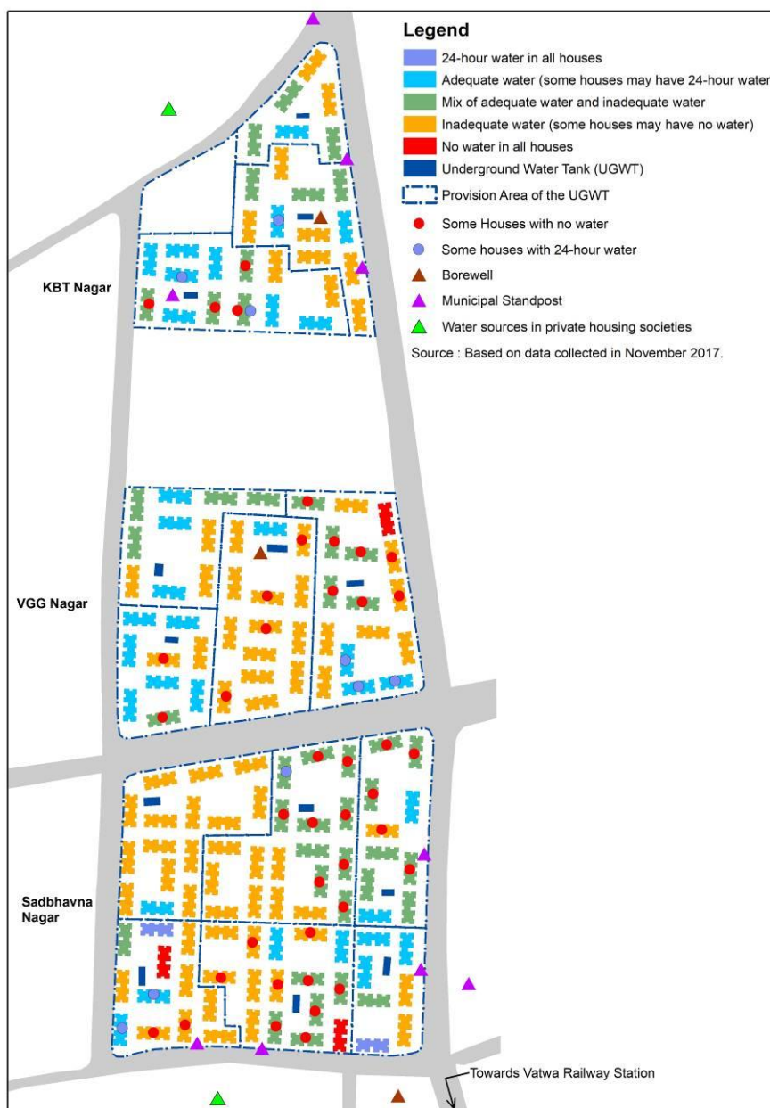
Figure 3. Water infrastructure and water conditions at the sites in November 2017 (Map by Vishal Darji).
