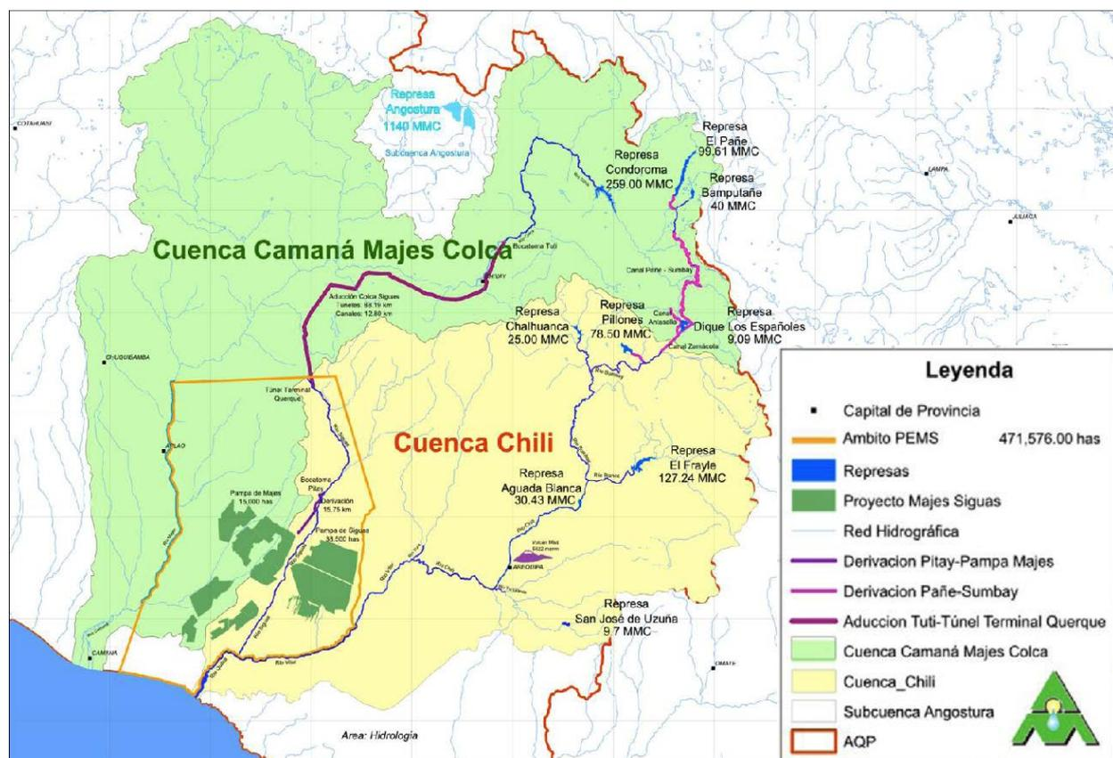
Note: The map shows how water is transferred from the Camaná-Majes-Colca basin to the Quilca-Chili via infrastructure at two points (purple). The southeastern part of the Quilca-Chili basin, the non-regulated Chili, is supplied by springs, aquifers and a small reservoir (Represa San José de Uzuña) with a storage capacity of 9.7 Mm<sup>3</sup> (Source: AUTODEMA).
