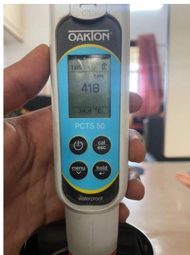
Figure 2. A TDS meter is used to show the quality of output from an RO water purifier.
